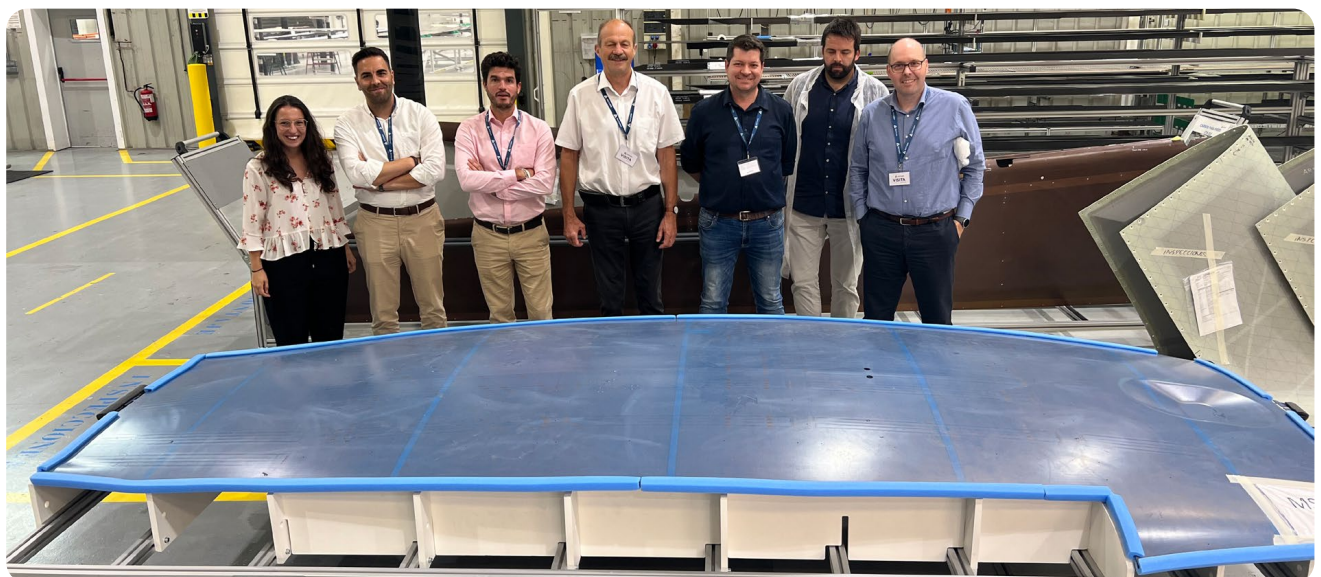
The first composite section belly skin of the Lilium Jet was completed in July 2023.
