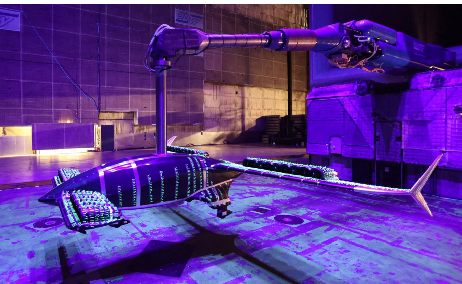
A first wind tunnel test campaign, using a complete Lilium Jet model was completed in June 2023
