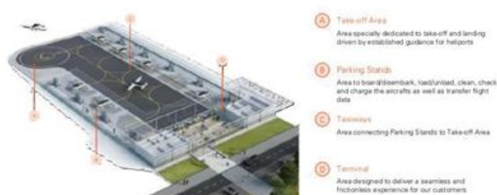
Lilium vertiports are based on a modular design and consist of four modules
