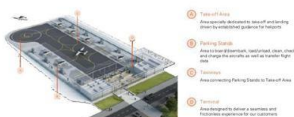
Lilium vertiports are based on a modular design and consist of four modules
