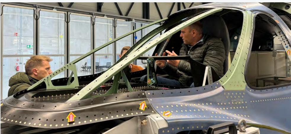
Trial fitting of pilot seat built by French supplier Expleseat
