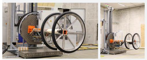
Propulsion test facility with a double propulsion unit
